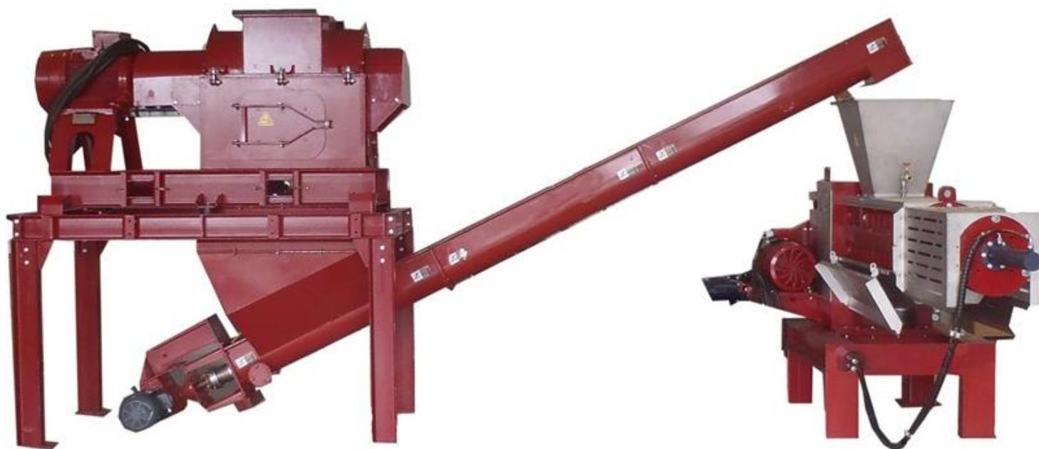
**Function :** producing a clean organic product suitable for biogas installations by separating the organic material from the packaging.
