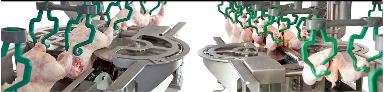
The breast cap cutter gives an exactly positioned, constant and symmetrical cut. This allows for a maximum of valuable breast meat to be left with the cap while minimizing bone contamination of untrimmed filets in the form of ribs. The module can cut the ribs at variable lengths. The module is placed after the HY wing cutter.
